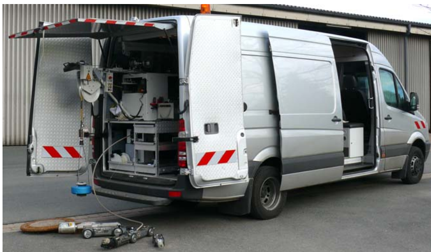
Fig. 4 - 6 Inspection van with inspection cameras
